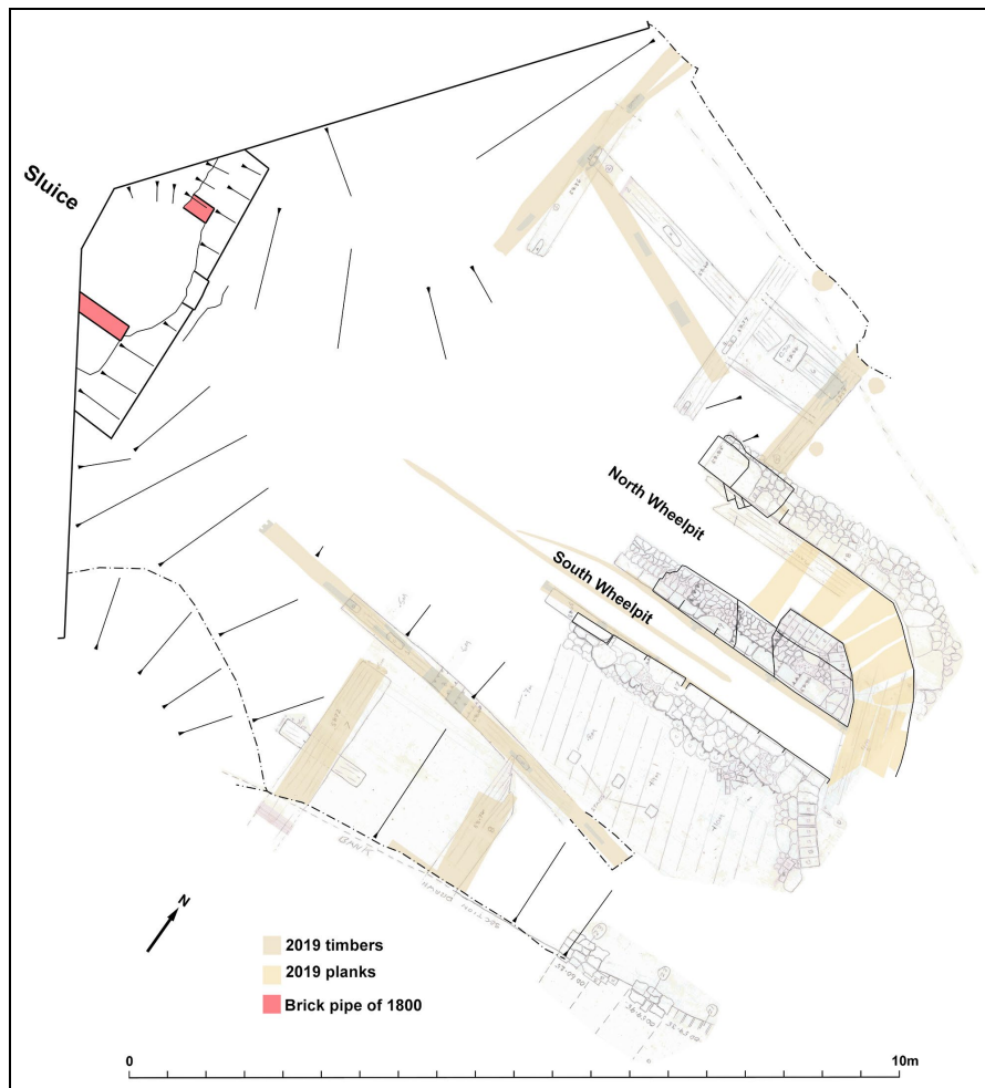
Figure 5 Plan of the sluice works
